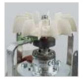
Motor with encoder technology and fan assisted ventilation, to guarantee intensive use
