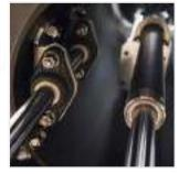
Linear guide system with chrome-plated steel cylinders
